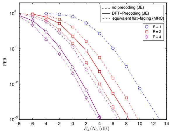
Fig. 8. Phase-precoding performance over the SCME channel model using the DFT-based precoding solution with period  $P = 4$ .
