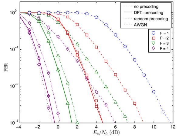
Fig. 5. FER performance of the precoded HARQ system over long-term quasi-static frequency-selective channel ( $\rho = 1$ ) using QPSK modulation. The receiver was implemented using the joint equalization scheme without turbo-iteration.
