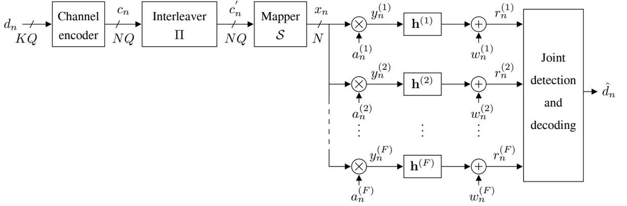
Fig. 1. Phase-precoded HARQ system model.
