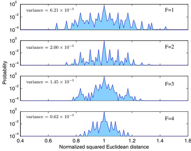
Fig. 2. Normalized squared Euclidean distance distribution at the output of the Proakis-C ISI channel for input error sequences of length  $N = 600$  of Hamming weight  $w = 10$  using BPSK modulation and bipolar precoding alphabet for  $F = 1, 2, 3$  and 4.
