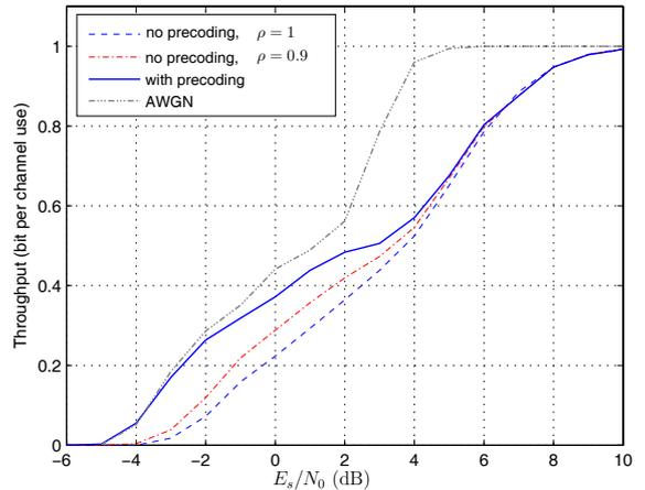
Fig. 6. Throughput of precoded HARQ system over correlated frequency-selective channels for various values of channel correlation coefficient  $\rho$  using the DFT-based precoding solution of period  $P = 4$  and QPSK modulation.
