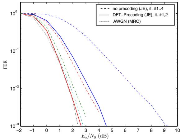
Fig. 7. Convergence behavior of the MMSE turbo-equalizer for the precoded HARQ system over a long-term quasi-static frequency-selective channel using the DFT-based precoding solution of period  $P = 4$  and QPSK modulation.
