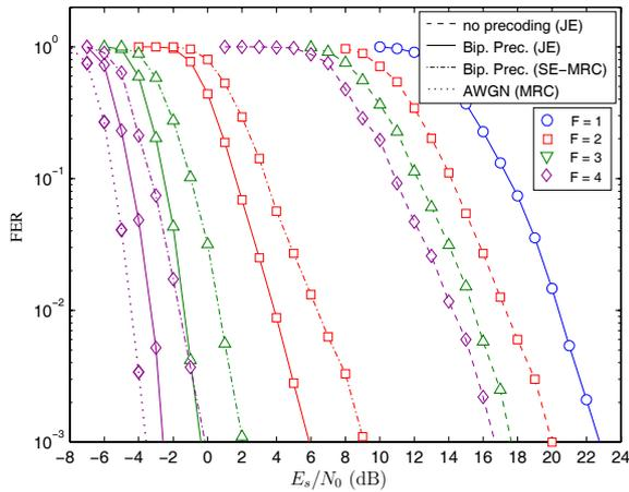
Fig. 4. FER performance of the precoded HARQ system over the Proakis-C frequency-selective channel using BPSK modulation and joint MMSE equalization without turbo-iteration.
