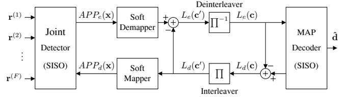
Fig. 3. Turbo-equalizer structure.
