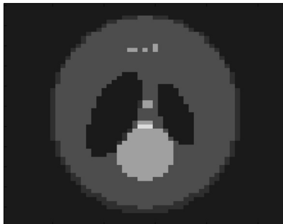
Fig. 11. Shepp–Logan phantom reconstruction without collimator.
