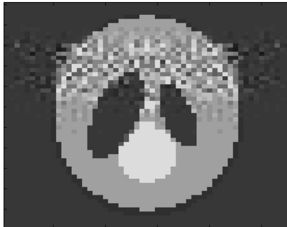
Fig. 10. Shepp–Logan phantom reconstruction with collimator.
