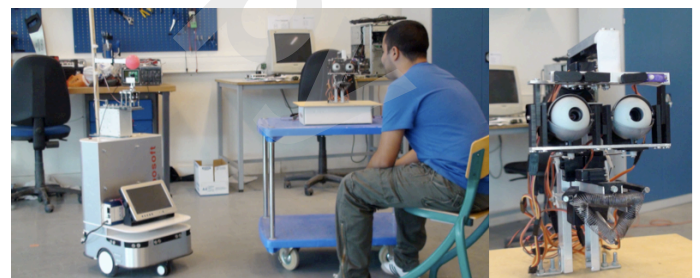
Figure 9. Experimental set-up: a robotic head that learns facial expression recognition and a mobile robot able of autonomous visual navigation tasks learning. The room size is 7m x 7m, but the robot's movements are restricted to an area of 3m x 3m (to allow a good video tracking of the robot's trajectories).
